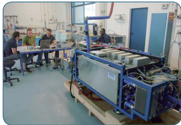
The ZEMships fuel cell system on the test bench at Proton Motor (May 2008).
